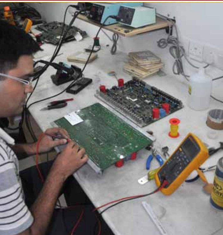
PCB repair shop in the new Picanol Indian headquarters
