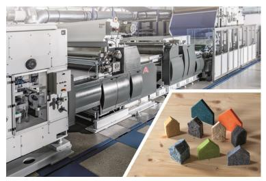
At the heart of the system is a state-of-the-art scanner that meticulously evaluates the weight distribution of the finished product. This critical data is used as the basis for real-time adjustments in the crosslapper and card infeed section, ensuring remarkably consistent distribution of the carded web.
