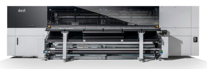
Light barriers at the infeed and outfeed as well as an all-round protection system ensure the necessary production safety for personnel and machine. The high-speed version P5 350 HS with a maximum printing speed of 700 m2/h, which is more than double compared to the standard model, in combination with Durst Automat and the corrugated option, is the ideal solution for entry-level digital corrugated printing for the packaging and display sector.
