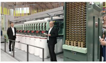
The highlight is the new air-jet spinning machine J 70. It enables spinning mills to achieve an unprecedented low level of production costs per kilogram of yarn, coupled with high flexibility and reliability. In combination with high productivity, the unique yarn
