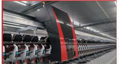
Starting with our new Autocard SC7, for example: all drafting systems are driven independently and can be adjusted easily online to facilitate processing of recycled fibres. Increasing the carding area to over 4m<sup>2</sup> makes it possible to gently process all fibre types and results in productivity.
