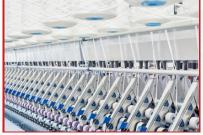
The integrated chute feeder ensures continuous, even feeding and sliver quality; Each drafting unit is driven independently which means online process adjustment is easy and the card can easily cope with recycled fibres. Dropping detection and automatic settings improve the utilization rate of fibre material and increase profitability for our customers. Our rotor-spinning machines are ideal for processing recycled fibres with a high short-fiderexcoente no READ THE FULL ARTICLE
